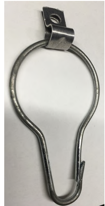
Mount it with the top of the big loop on any surface so that it can swivel a bit back and forth. Like this.
