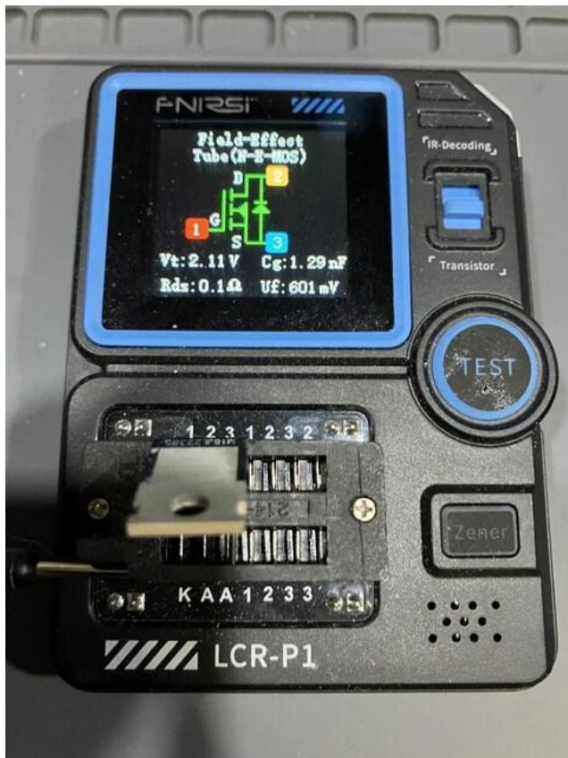
Remove both transistors. One of them is still good - the tester shows this-
