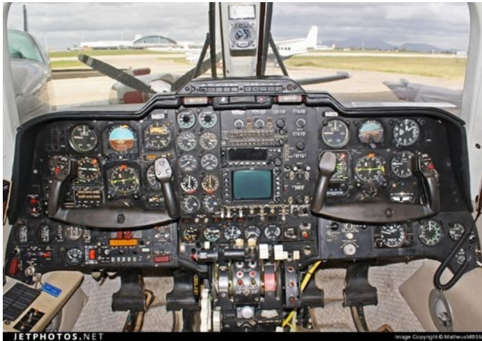
The cockpit was complicated, having over 240 toggle switches, pushbuttons, knobs, dials, and meters.
