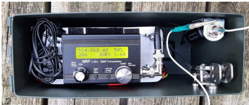
Usable SWR with the tunerless Emergency Field Antenna for 20m hooked up to a QMX
