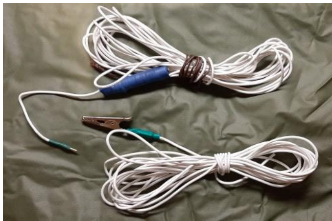
The Emergency Field Antenna for 20m. Note the radiator wire (top) uses a simple BNC center pin to connect to the radio. The blue component is the loading coil. The bottom wire is the counterpoise. Both 26awg wires are 13ft long.
